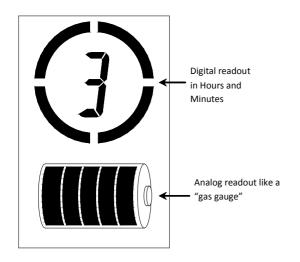
The RealTime<sup>™</sup> LCD provides on-the-fly remaining run time estimates in 15 minute increments as well as providing remaining capacity information using the traditional "gas gauge" approach. In this way, the LCD provides two different methods of determining battery capacity.
