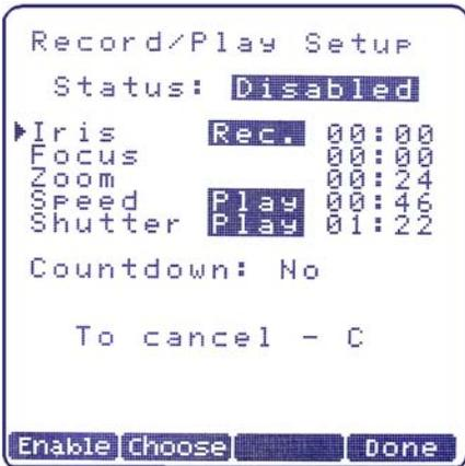
fig.7 Record/Playback Setup
