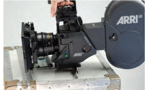
Finding the camera's fore-aft center of gravity.
