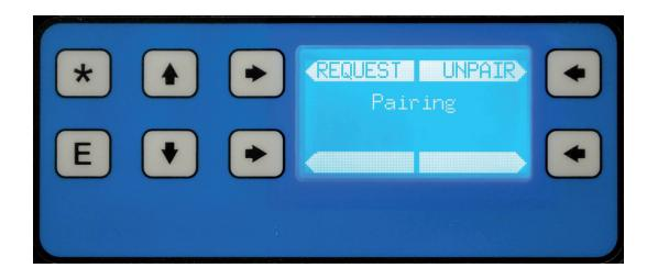
Pairing is only used in Unicast mode. It offers 256 AES Encrypted one transmitter to one receiver transmission.
