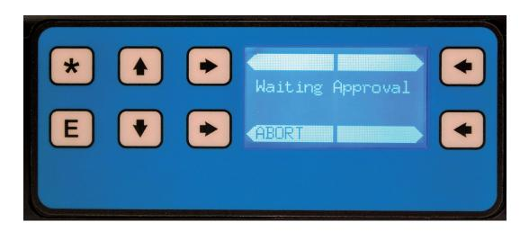
When the receiver has located the transmitter, the transmitter ID will appear on the receiver's LCD screen. At this point you have the option to either "Approve" the pairing, or "Reject" the pairing if the transmitter ID does not match the transmitter that the receiver is to be paired with.
