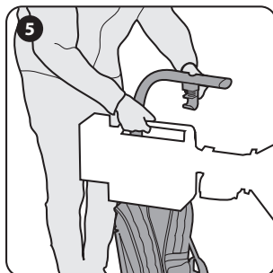
Fig. 3 With the Easyrig VARIO 5 firmly sitting on ground, attach the camera to the hook. Check to make sure the camera is supported properly. • If the tension is incorrect to support your camera weight, continue to step 4a. • If the tension is correct to support your camera weight, continue to step 6.
