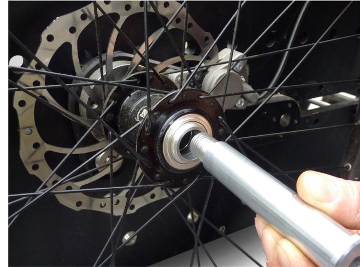
To remove the wheels, jack up the *RICKSHAW DOLLY*®. Hold the wheel in place and loosen the wheel bolt with a Size 8 Allen wrench.
